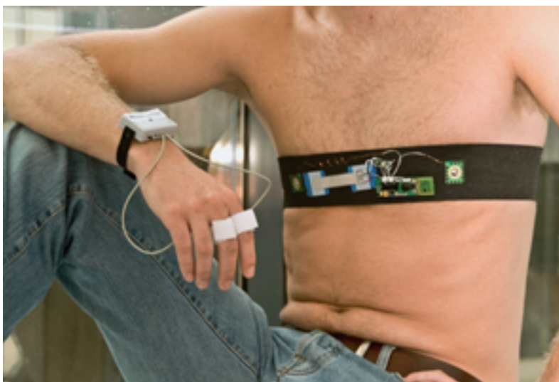
The wireless body environment network measures physiological signals and analyses them in real time
