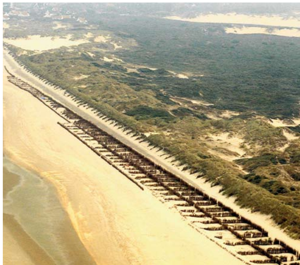
The planting of "beach hedges" of tough grasses on the dunes helps retain sand and protect against erosion
