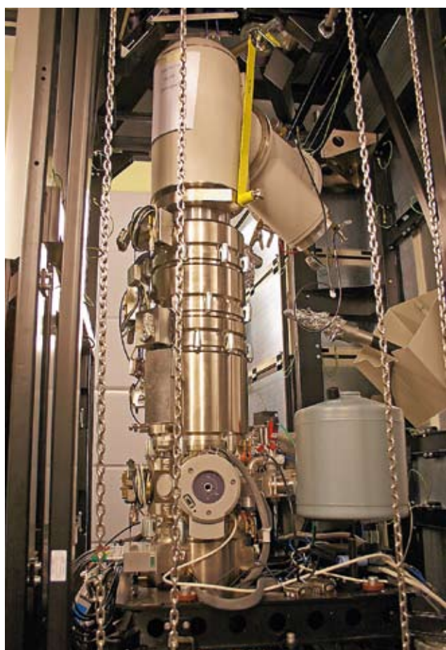
The Qu-Ant-EM can distinguish details of 50 picometres, or one-trillionth of a metre
