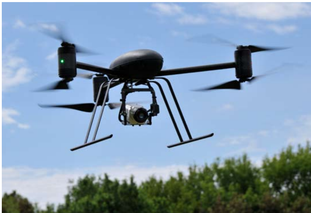
A hyperspectral camera attached to a remote-control helicopter can help fight fires
