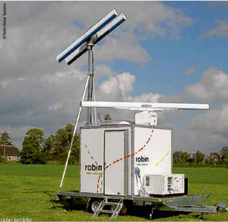
This radar can automatically detect every bird within a distance of 10 kilometres and even recognise the species
